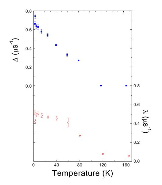
Fig. 4.4: Temperature dependence of the relaxation rates  $\Delta$  (solid squares) and  $\lambda$  (open circles) from Eq. (4.1).
