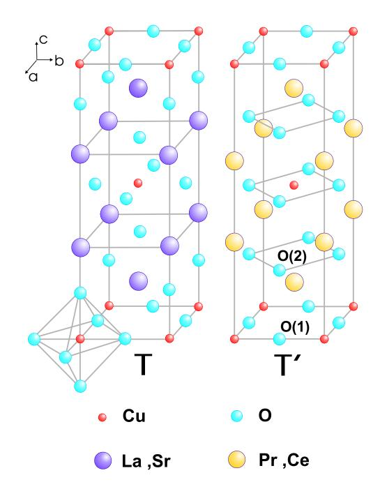
Fig. 3.1: Crystal structure of  $La_{2-x}Sr_xCuO_4$  and  $Pr_{2-x}Ce_xCuO_4$ .
