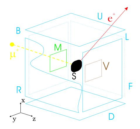
Fig. 2.2: Schematic diagram for a typical TD- $\mu$ SR experiment. The  $\mu$ SR coordinate system convention is also shown at the lower left.
