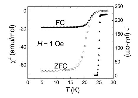
Fig. 3.2: Bulk magnetic susceptibility measurements taken under field-cooled (FC) and zero-field cooled (ZFC) conditions with H = 1 Oe and resistivity measurements (solid triangles) in zero external magnetic field. The applied field is directed along the crystallographic  $\hat{c}$ -axis.
