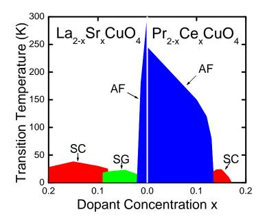
Fig. 1.1: Generic Phase diagram of the hole-doped HTSC  $La_{2-x}Sr_xCuO_4$  and the electrondoped HTSC  $Pr_{2-x}Ce_xCuO_4$  as a function of charge doping concentration, showing the anitferromagnetic (AF), spin glass (SG) and superconducting (SC) phases.
