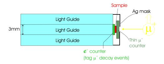
Fig. 3.3: Schematic of the experimental setup. All the components are contained within a <sup>4</sup>He gas-flow cryostat.
