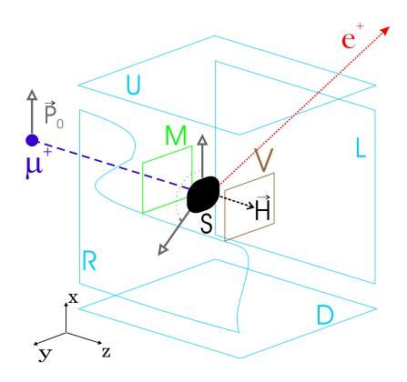
Fig. 2.3: Schematic diagram of a TF- $\mu$ SR experiment. The initial muon spin polarization  $\vec{P}_0$ , indicated by the open arrow at  $\mu^+$ , is rotated by 90° so that it is perpendicular to the direction of the external magnetic field  $\vec{H}$ . The open arrows at the sample **S** illustrate the Larmor precession of the muon spin.
