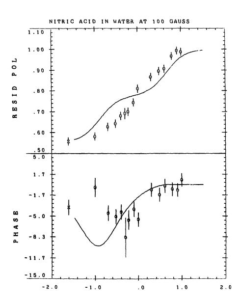
Figure 18 - HNO<sub>3</sub> at 100 gauss: Fit Assuming Proper Muonium Mechanism
